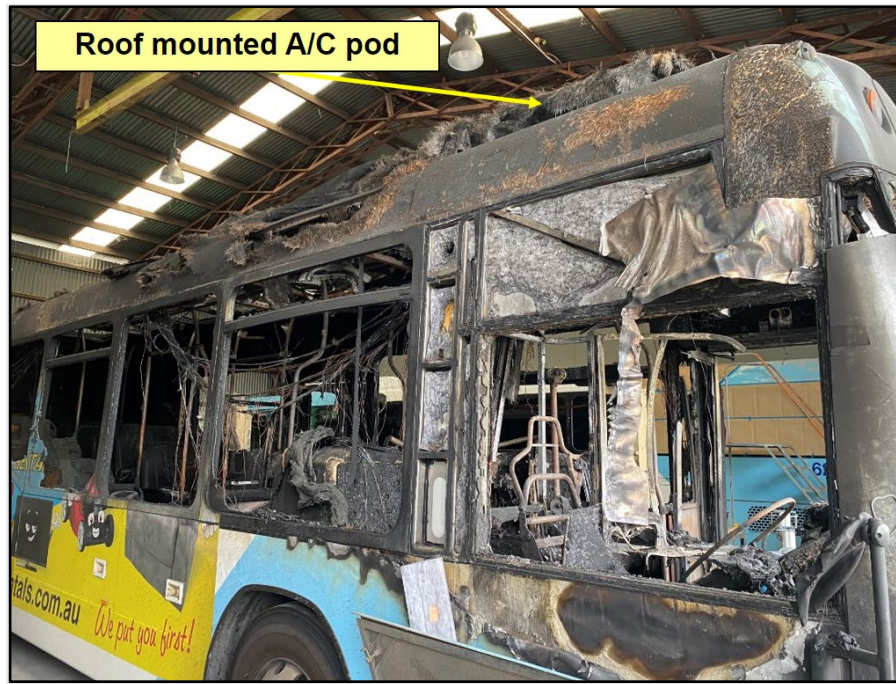
Figure 15: MO5103 fire damage on offside
