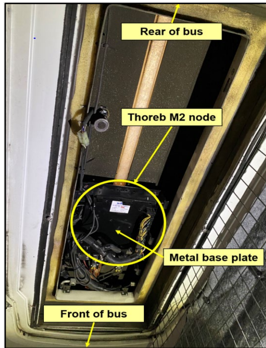
Figure 6: Roof location of Thoreb M2 Node in A/C system (in normal operating position with grill open)
