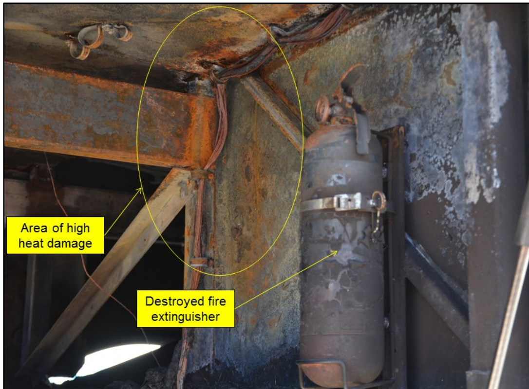
Figure 2: Fire damaged engine bay and extinguisher
