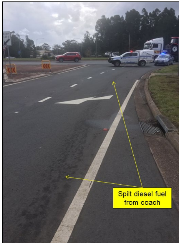
Figure 9: Diesel fuel leak leading to rear of coach
