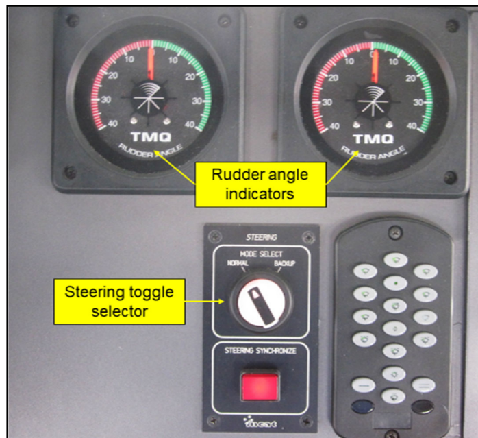
Figure 9: Primary/back-up toggle selector panel in detail
