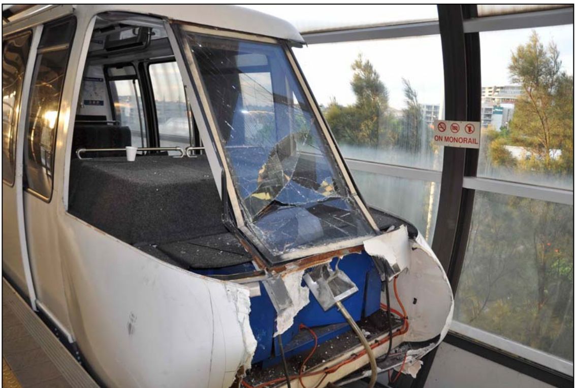
Photo 4: Collision damage to Monorail 4
