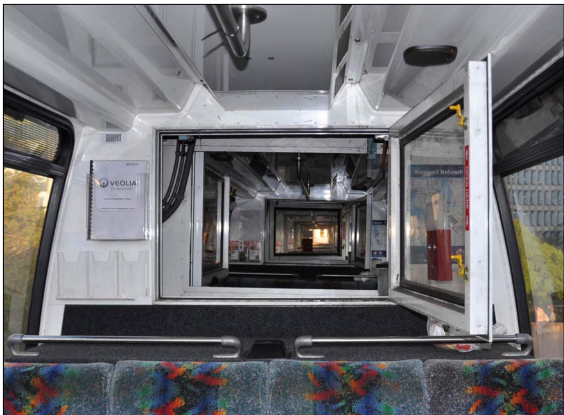
Photo 3: Emergency access window between monorail carriages
