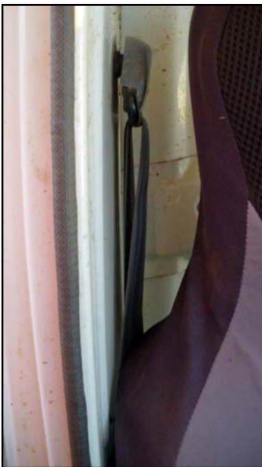
Photograph 11: Seat belt retracted and jammed behind seat back
