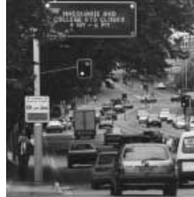
VARIABLE MESSAGE SIGNS CONTROLLED FROM THE TMC INFORM MOTORISTS OF CHANGING TRAFFIC CONDITIONS
