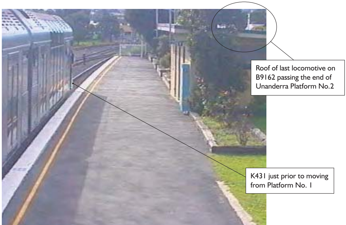
CCTV footage indicating that K431 had not departed Platform No.1 until both Locomotives on B9161 had passed the end of Platform No.2.
