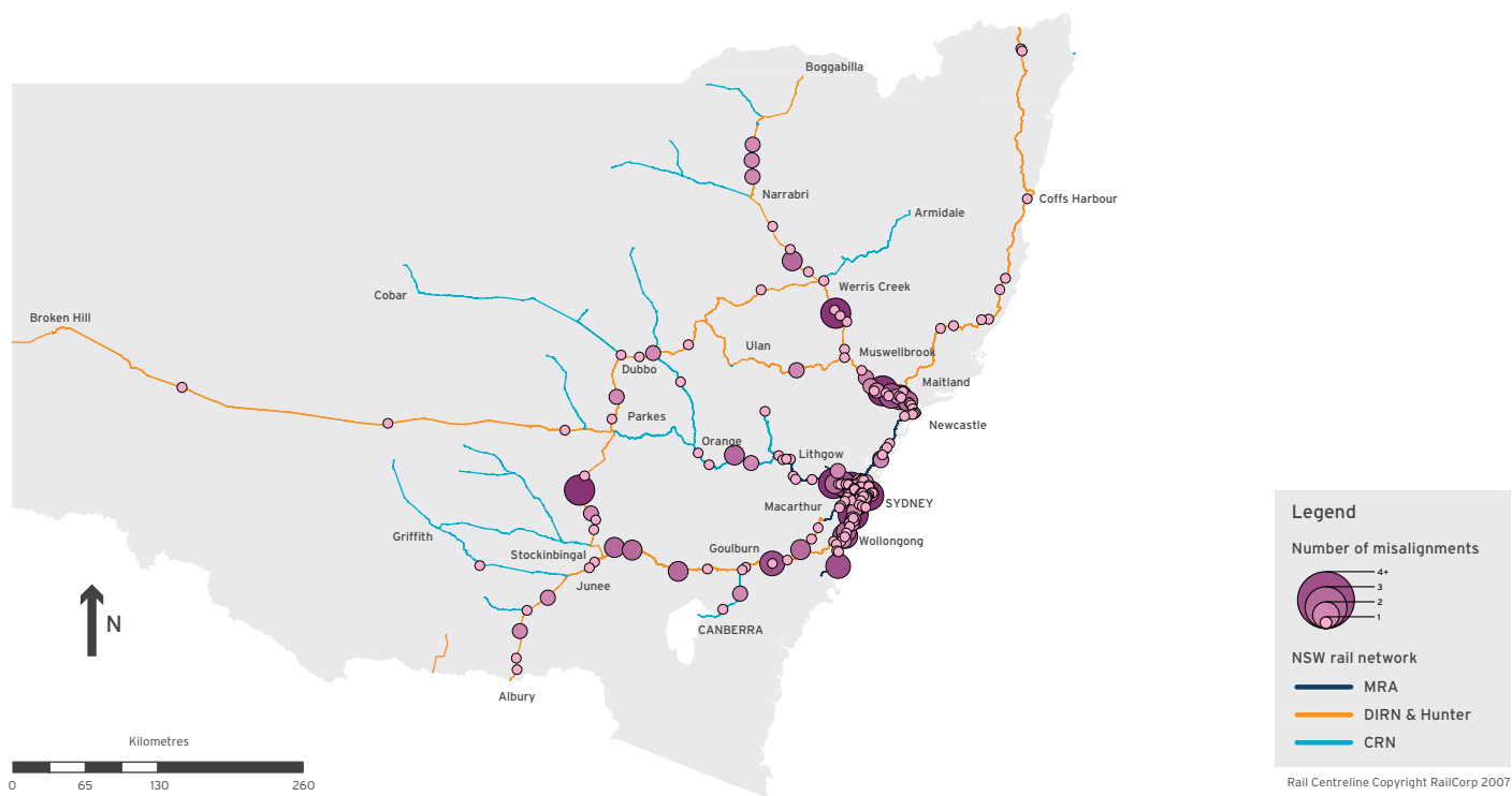
► Figure 47b: Misaligned track (running line) across the NSW rail network, 2008-09
