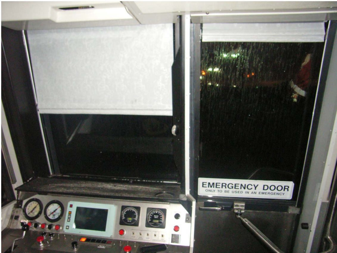
Photo 7: Drivers blind position on the windscreen and the emergency door
