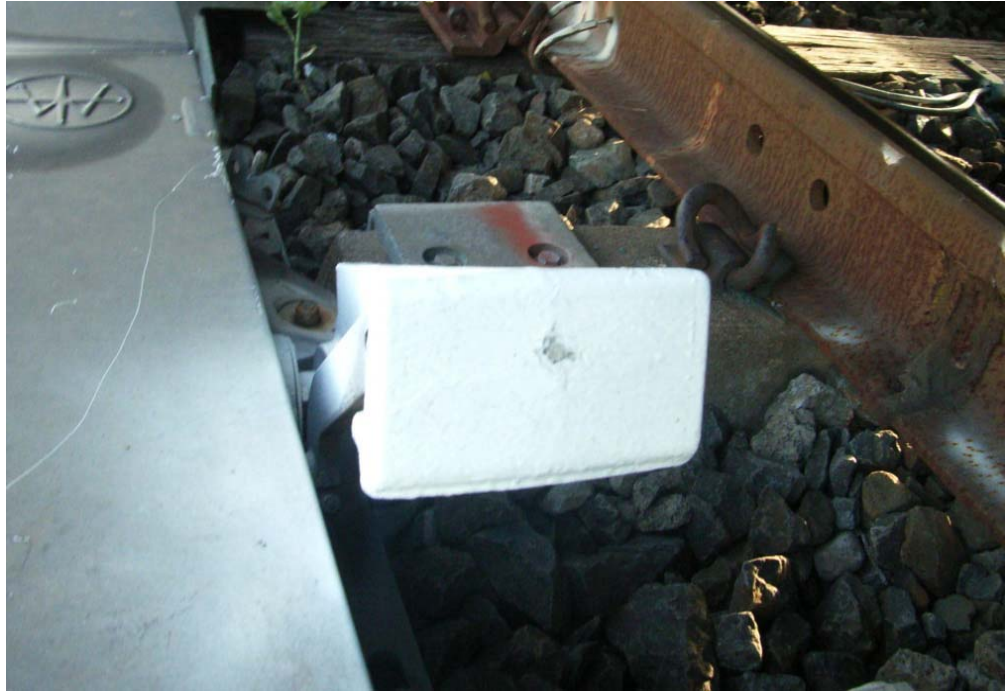
Photo 6: Train stop arm at Signal WG1010 showing a fresh strike mark from the trip gear of K496
