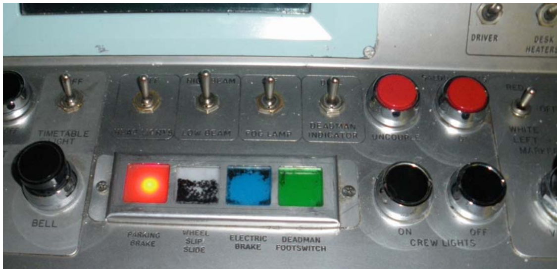
Photo 14: Drivers console on another Tangara service showing lenses coloured in
