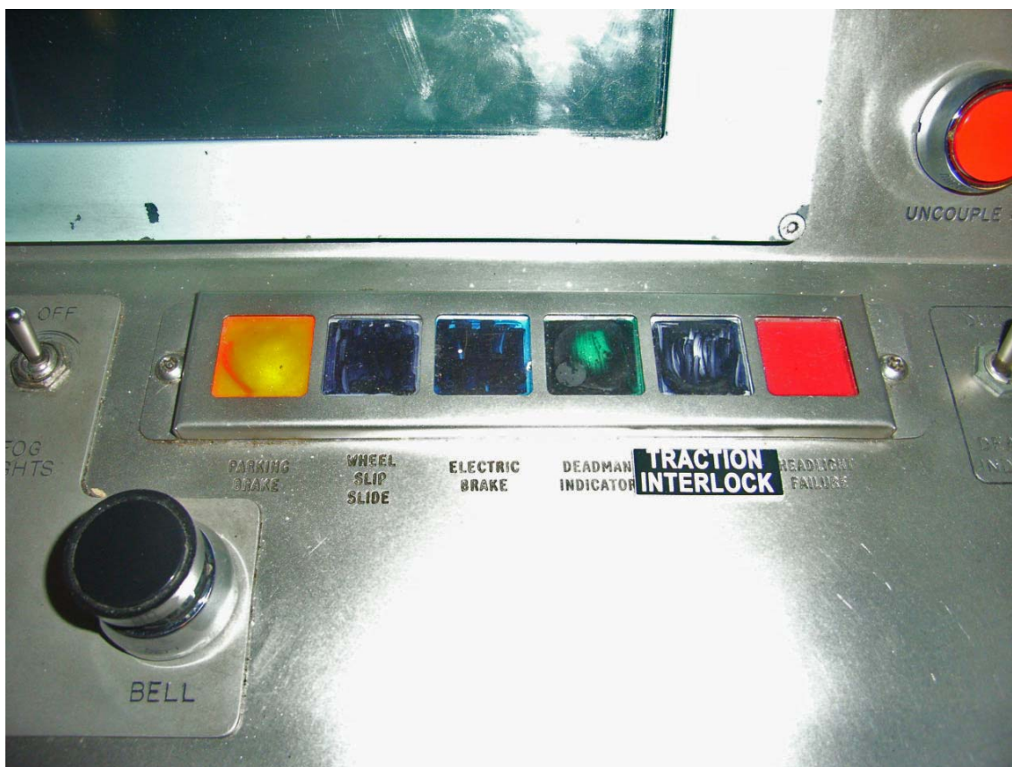
Photo 13: Drivers console on K496 showing lenses coloured in
