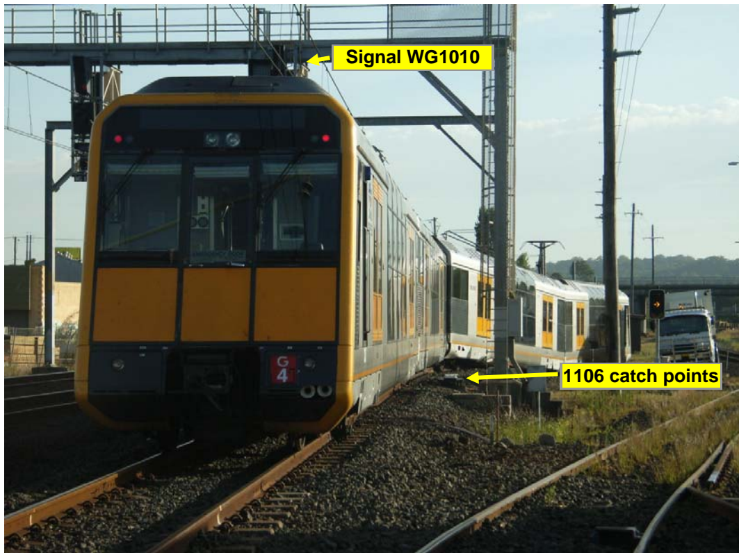
Photo 2: K496 showing front two cars derailed
