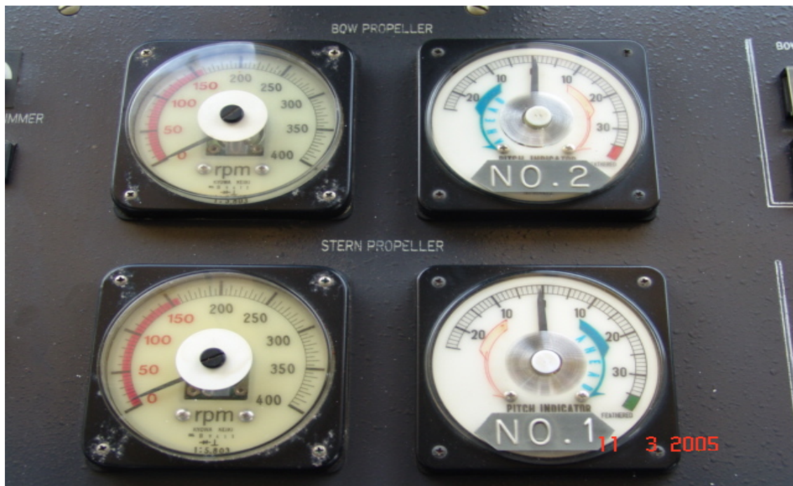
Figure 8: Gauges, available to a master, indicating pitch settings
