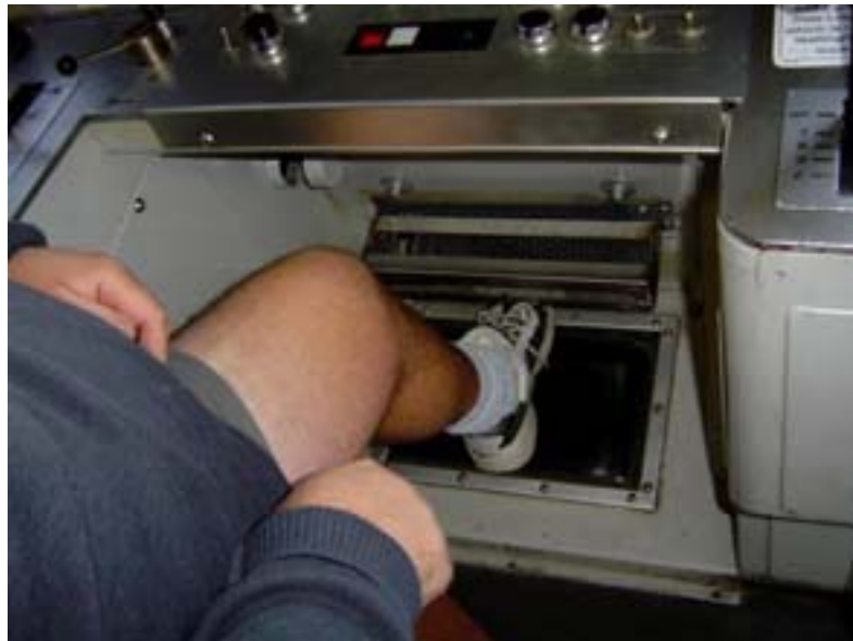
Picture 9: View of deadman system being operated, without effort, by the weight of a seated driver's leg. Note: this train was under way at the time of the photo. Also note proximity of the heater to the top of the driver's foot.
