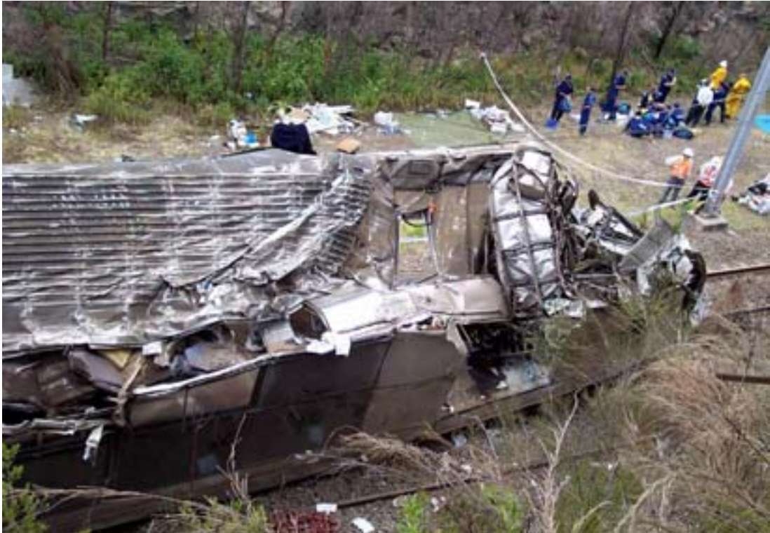
Picture 3: Impact damage to the first carriage.
