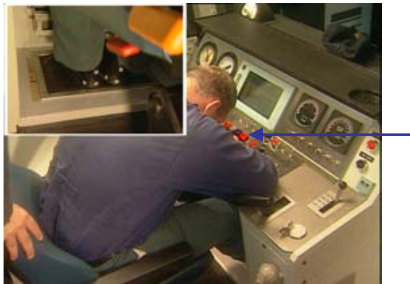
Picture 12: Driver feigning incapacitation with both feet on the deadman pedal. Note arrowed light indicating that the deadman system was suppressed in these conditions.
