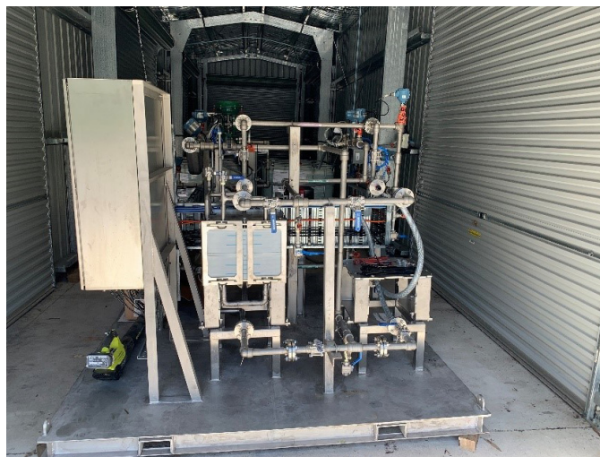
Experimental Forward Osmosis facility ready for acceptance testing at CSIRO in Pullenvale. Two Forward Osmosis modules shown on left hand side of skid. Photo courtesy of CSIRO.
