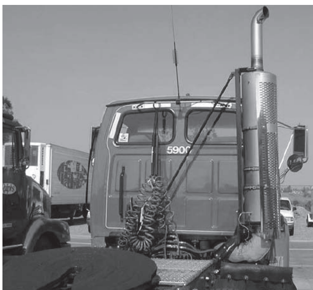
A diesel particle trap has been fitted to a truck as part of the Diesel Retrofit Program.
