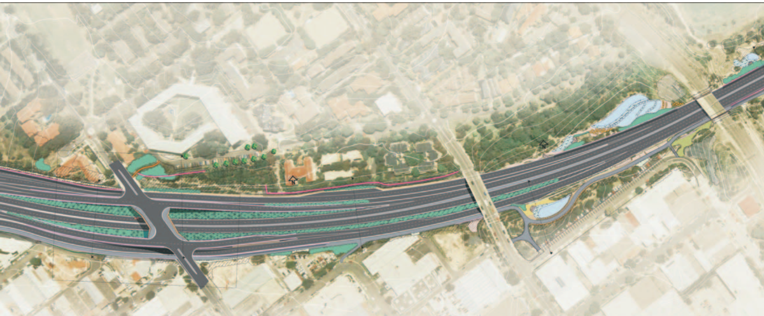
ramps and shared cycleway and pedestrian path between Nareburn and the eastern portals of the Lane Cove Tunnel and the Pacific Highway and Longueville Road (left).
