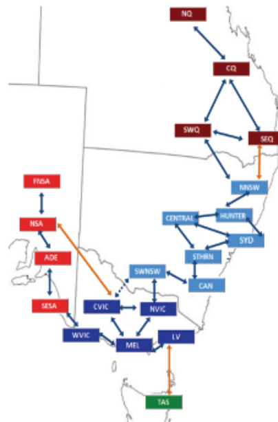
Figure 1: Map of the 21-node NEM transmission network simulated in the MUREIL scenarios. Orange lines represent HVDC links, while blue represents conventional HVAC. Dashed lines are under planning/construction.
