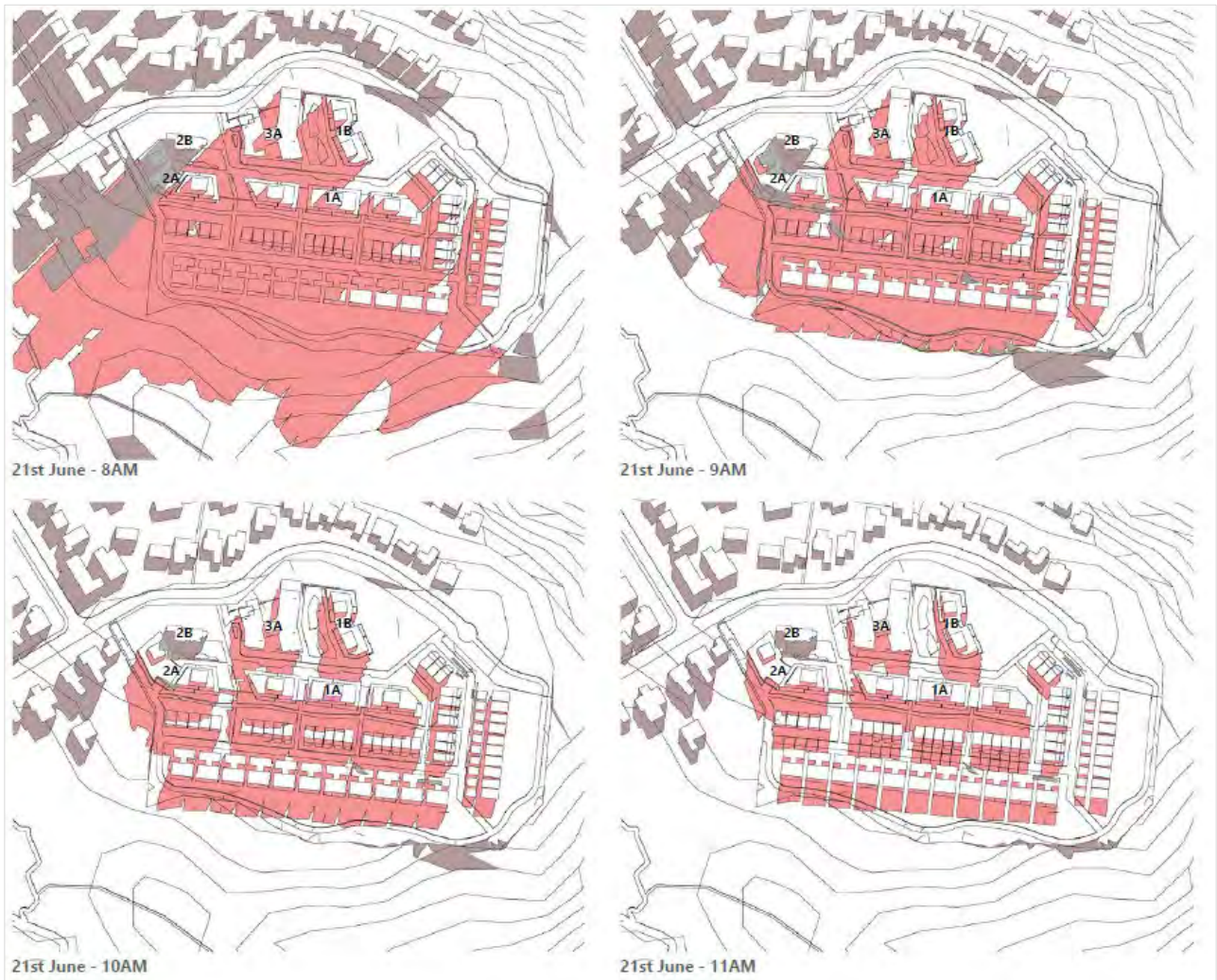
Figure 13 – shadow diagrams from planning proposal Urban Design Report - constant shadow from 5-7 storey buildings to central part of the site and dwellings
