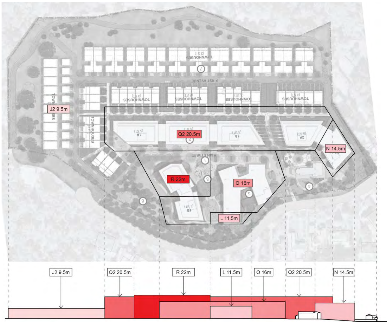
Above: Full street elevation and site plan of proposed maximum building heights.
