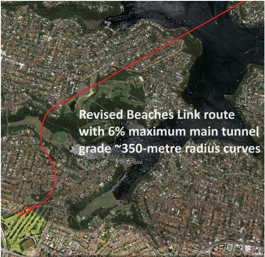
Figure 3: If the WHT is cancelled, the works at Cammeray can be repurposed as shown above for a Beaches Link with a ~6% main tunnel grade that is below the surface of the golf course.
