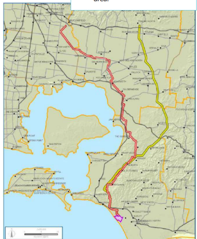
LEGEND Desalination Plant Site Boundary Current Transfer Pipeline Corridor Northern Grid Connection Corridor (500m) Municipality Boundary Highway Major Road Town Much of the transmission corridor located was along roadside easements where possible
