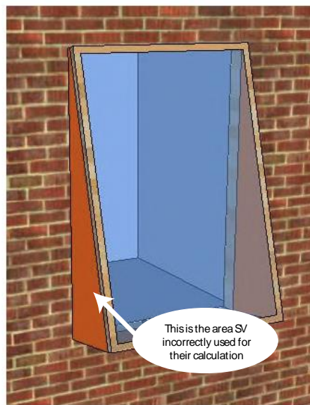
Figure 2b Incorrect area
