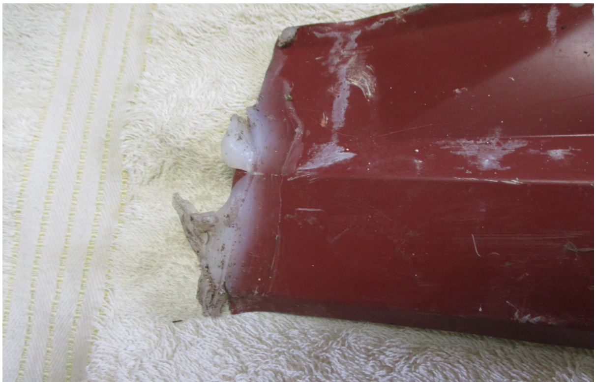
Edge of the red coloured side showing one of the glued joints
