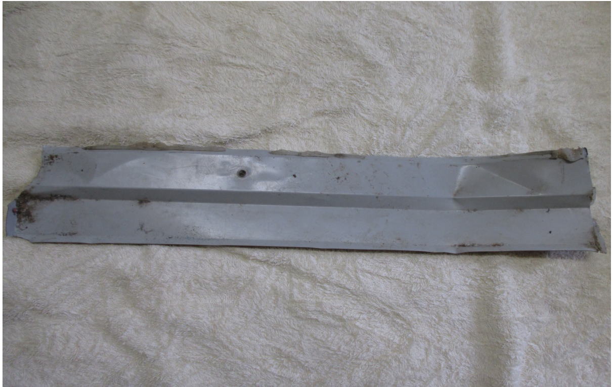
Reverse side of the steel sheet with broken glue line along the top edge
