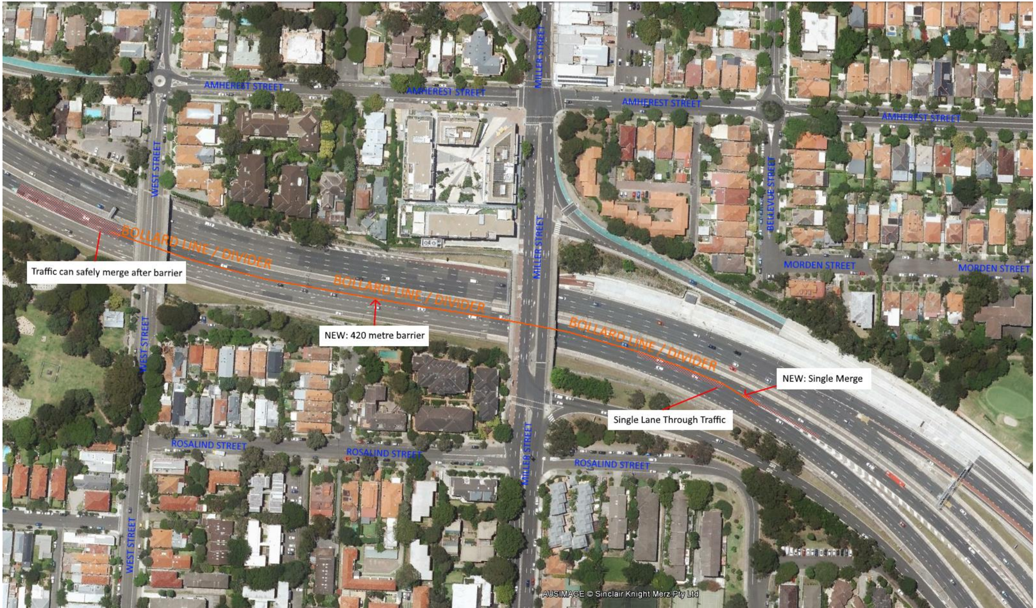
Figure 13: Warringah Freeway at Cammeray. Proposed solutions labelled and identified.
