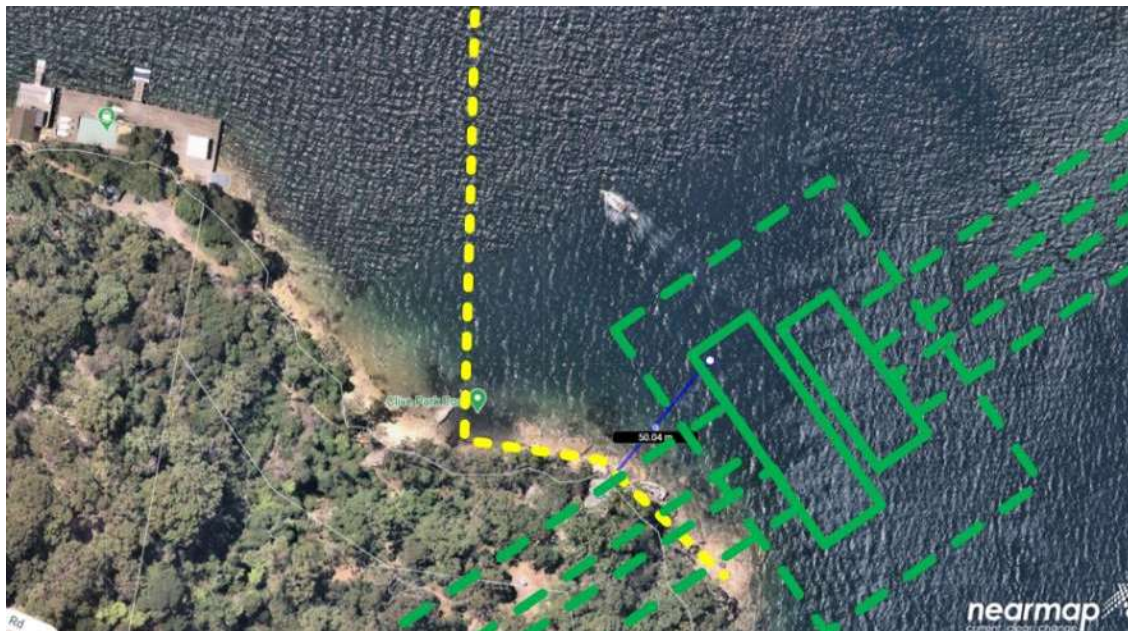
Figure 21 The proposed coffer dam works are located approx. 40-50m from Aboriginal shelter/cave (green), however the road header tunnelling works are located directly beneath the largest CPHA shelter/cave and rock art area.
