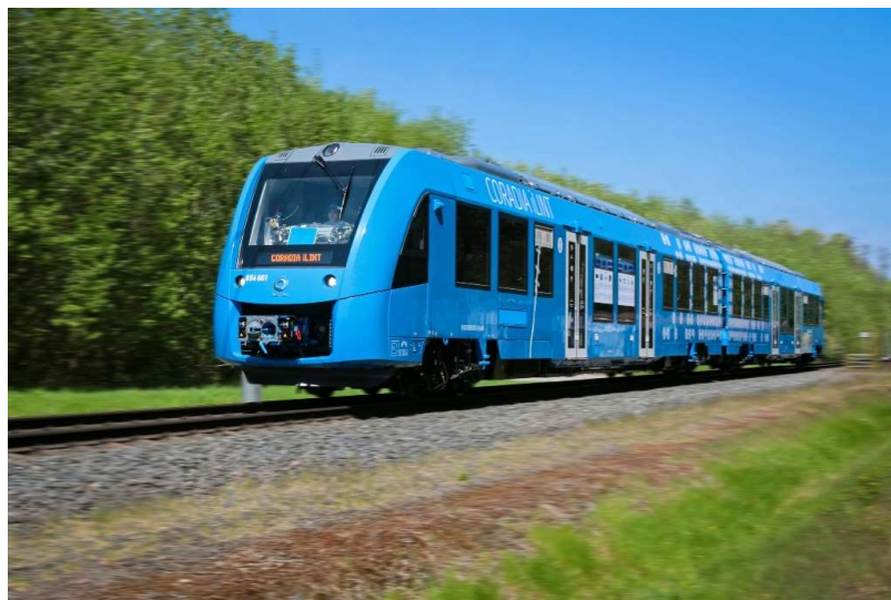
Figure 6: Alstom's Coradia iLint hydrogen passenger train, operative in Germany since 2018.
