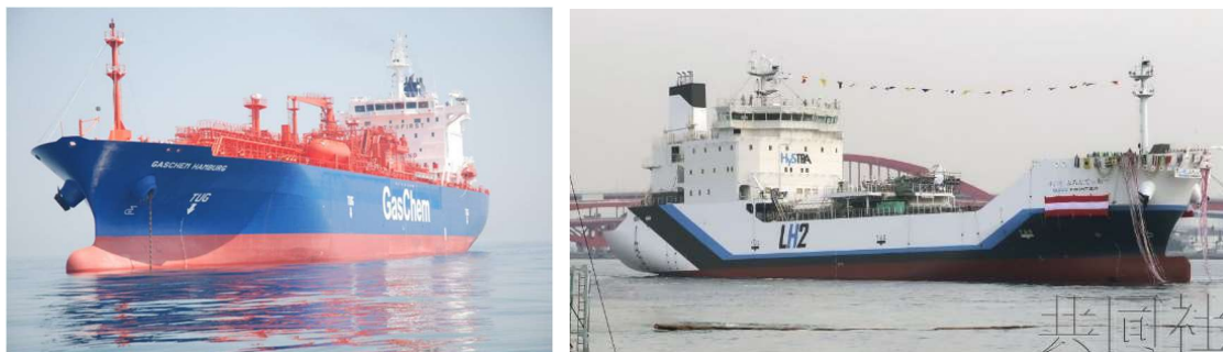
Figure 2: Left; conventional ammonia transport ship, Right; Suiso Frontier, the world's first liquefied hydrogen carrier, launched in Japan in December 2019.
