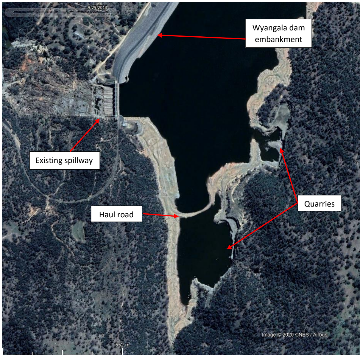
Figure 6 - Quarries used during construction of the existing Wyangala dam visible at low water levels (from Google Earth, image captured 29 September 2018). Reservoir level is 366.2m AHD (12.4m below FSL) or 656,000ML of stored water 18 . Wyangala total storage is 1,200,000ML.
