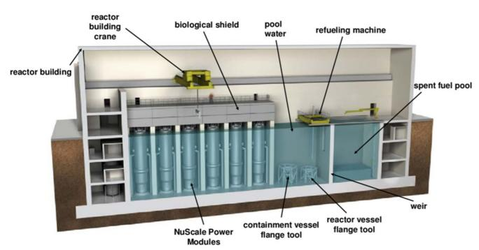
Figure 16. Cutaway of a NuScale "12-pack"  $^{\text{\tiny TM}}$
