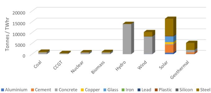
Figure 5. Material utilisation for plant construction for one TWhr energy. Source: US DOE "Quadrenniel Technology Review 2015", Table 10.4, pg 402
