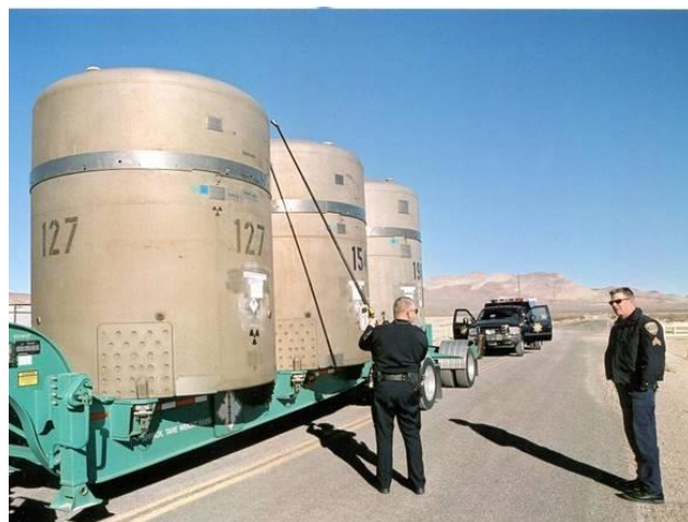
Figure 6. Highway Patrol Officers conduct radiological surveys and mechanical inspections on the first Nevada Test Site transuranic waste shipment at the Area 5 Radioactive Waste Management Complex located on the Nevada Test Site. These shipments travel on normal public roads to their final destination at the Waste Pilot Isolation Plant near Carlsbad, New Mexico. (source: NNSA)
