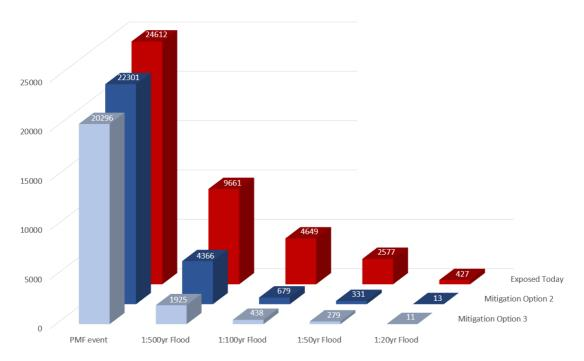
Under Mitigation Option 2, there is a **34% reduction** in the number of properties exposed to over-floor flooding.
