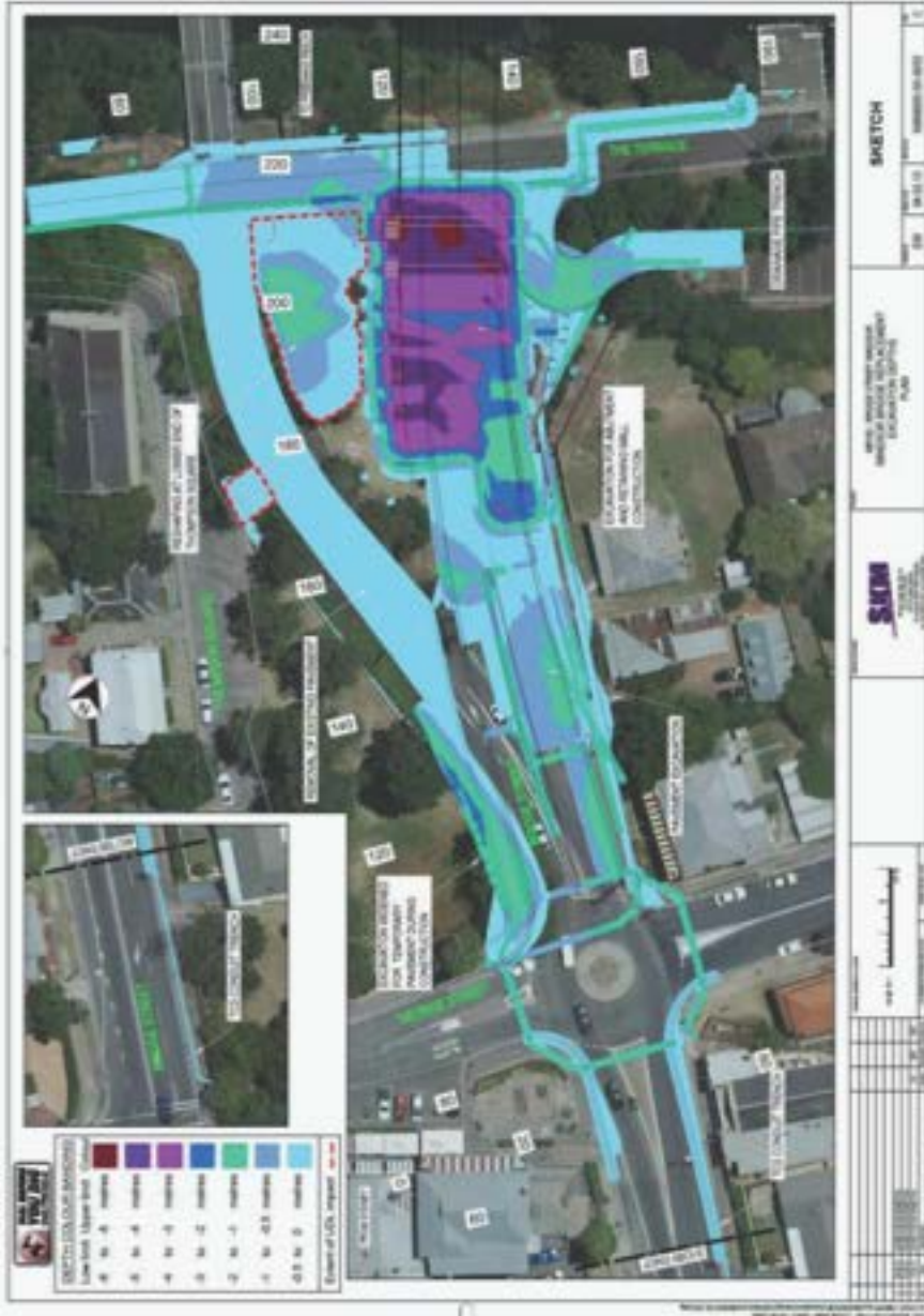
Plate 4: Diagram showing the depth of excavation in Thompson Square associated with the construction program. (Source SKM)
