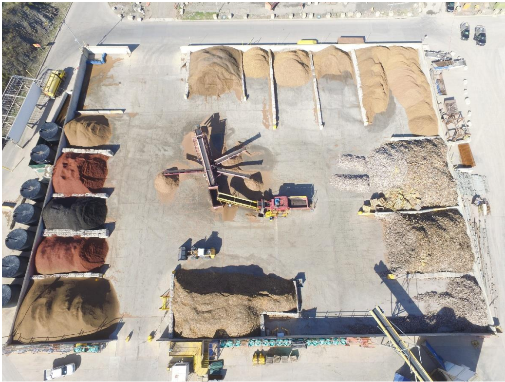
Figure 12: Recovered wood-waste material in the crushing and screening yard at Genesis Recycling Facility (Aggregates, sands, mulch)
