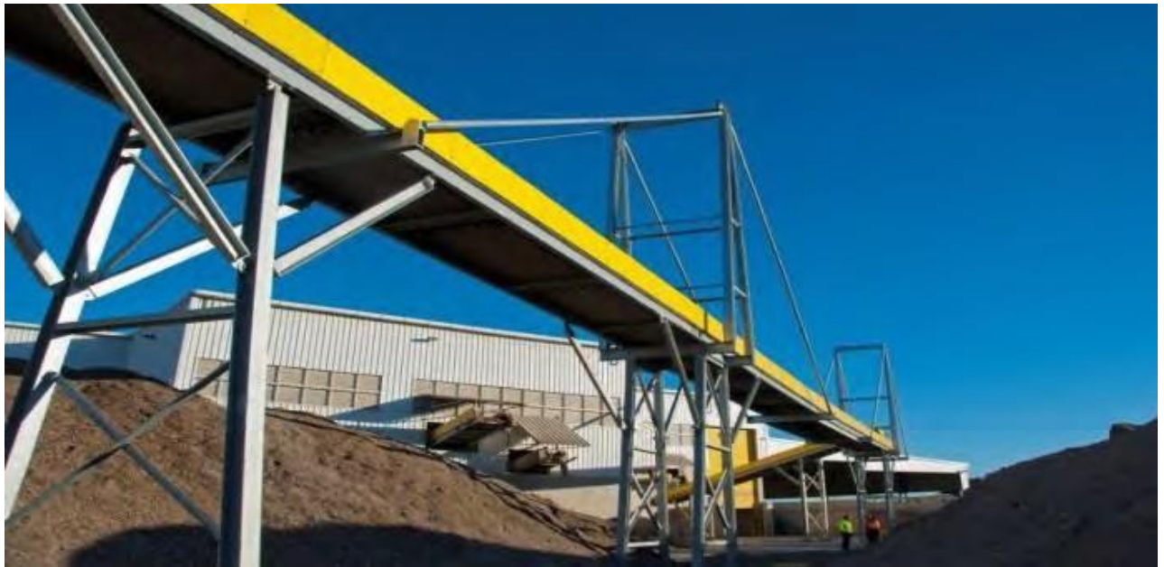
Figure 15: Electrically driven conveyors with sorting and screening technology at Genesis Recycling Facility
