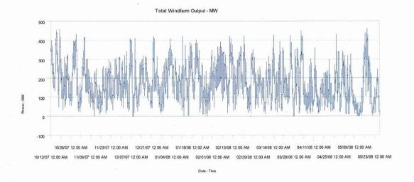
The graph shows quite clearly that, for windfarms in SE Australia, separated by distances of up to 1000 km, there is no appreciable smoothing of the output resulting from geographic dispersion.
