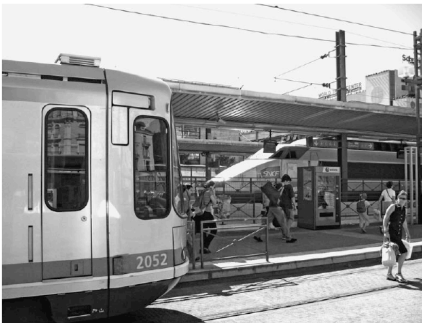
Seamless interchange between tram and TGV (high speed rail) at Grenoble (France), population 175,000 (smaller than the Newcastle urban area). The station design provides for parallel platforms, which is not possible at the Wickham site due to insufficient site width.
