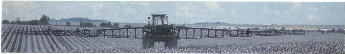
Photo 4 – JD 7760 Cotton baler modified to cover 12 metre double skip on 3 metre spacings with additional trailer to carry bales out of the field. Reduces compaction and traffic infield.
