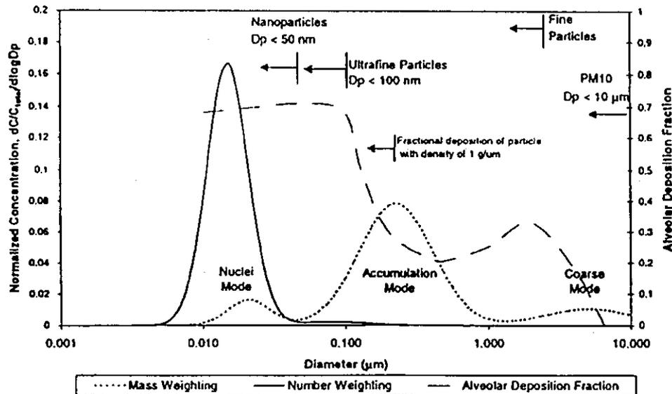
Typical engine exhaust mass and number weighted size distributions shown with alveolar deposition.
