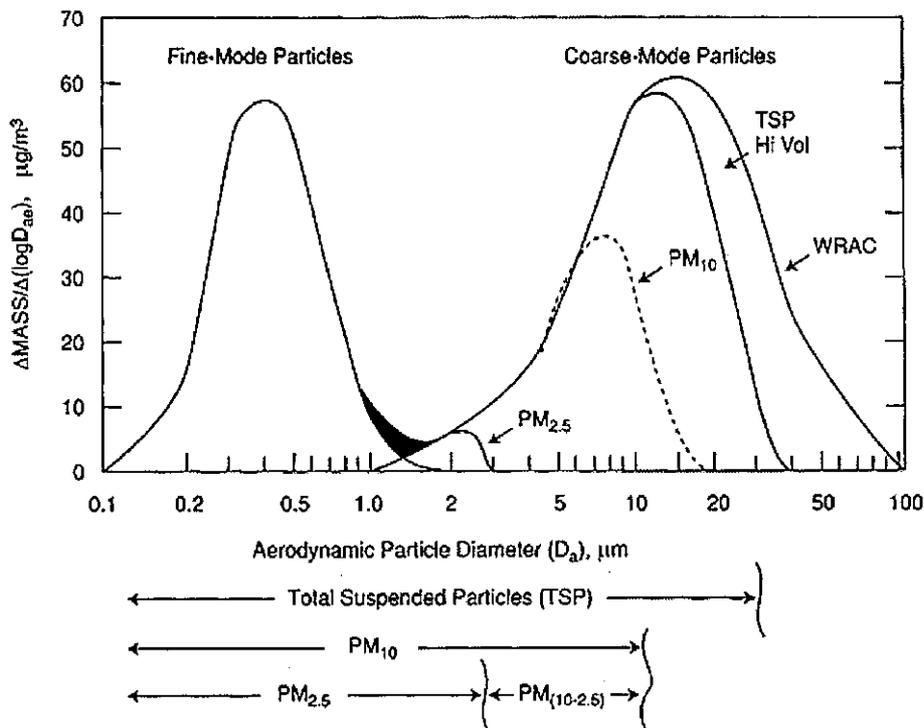
Figure 3. Representative example of a mass distribution of ambient PM as function of aerodynamic particle diameter. A wide-ranging aerosol collector (WRAC) provides an estimate of the full coarse mode distribution. Inlet restrictions of the high volume sampler for TSP, the PM<sub>10</sub> sampler, and the PM<sub>2.5</sub> sampler reduce the total mass reaching the sampling filter. Below is depicted a diesel particle with adsorbed PAH's on the surface
