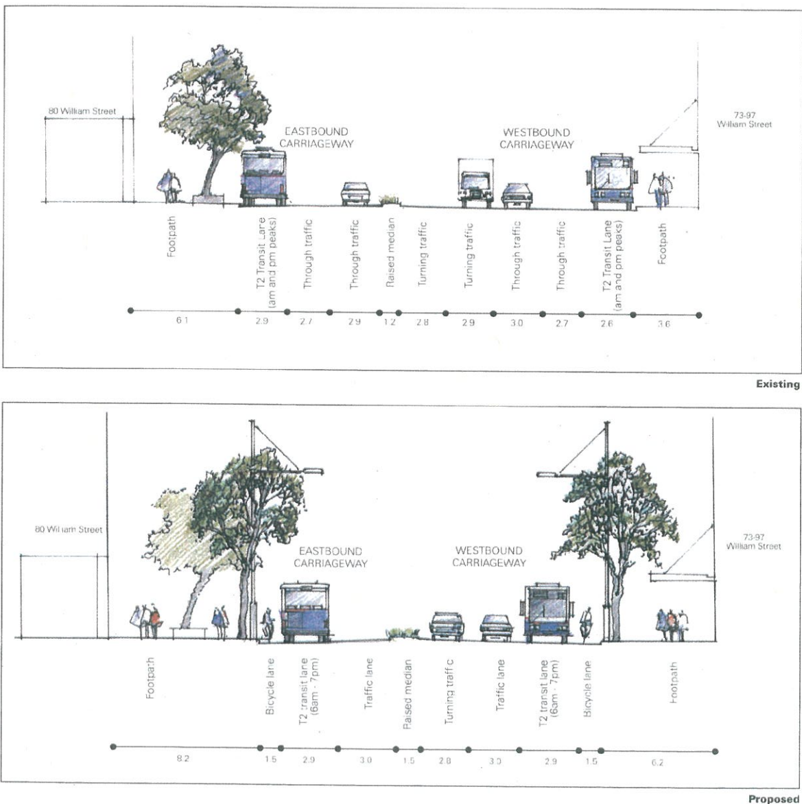
Figure 7.20 Cross-section of William Street between Crown Street and Riley Street: Existing and Proposed
