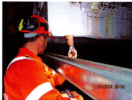
Conducting Ultrasonic test on one hanger
