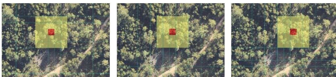
Figure A2.2: The process of pixel 'smoothing' using the focal majority approach, where the processing cell in red is attributed the majority value of all cells within the focal window identified in yellow
