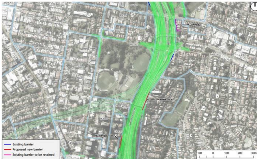
Figure 7-3 – Noise barriers considered in the NMG analysis at Warringah Freeway and surrounds (north)
