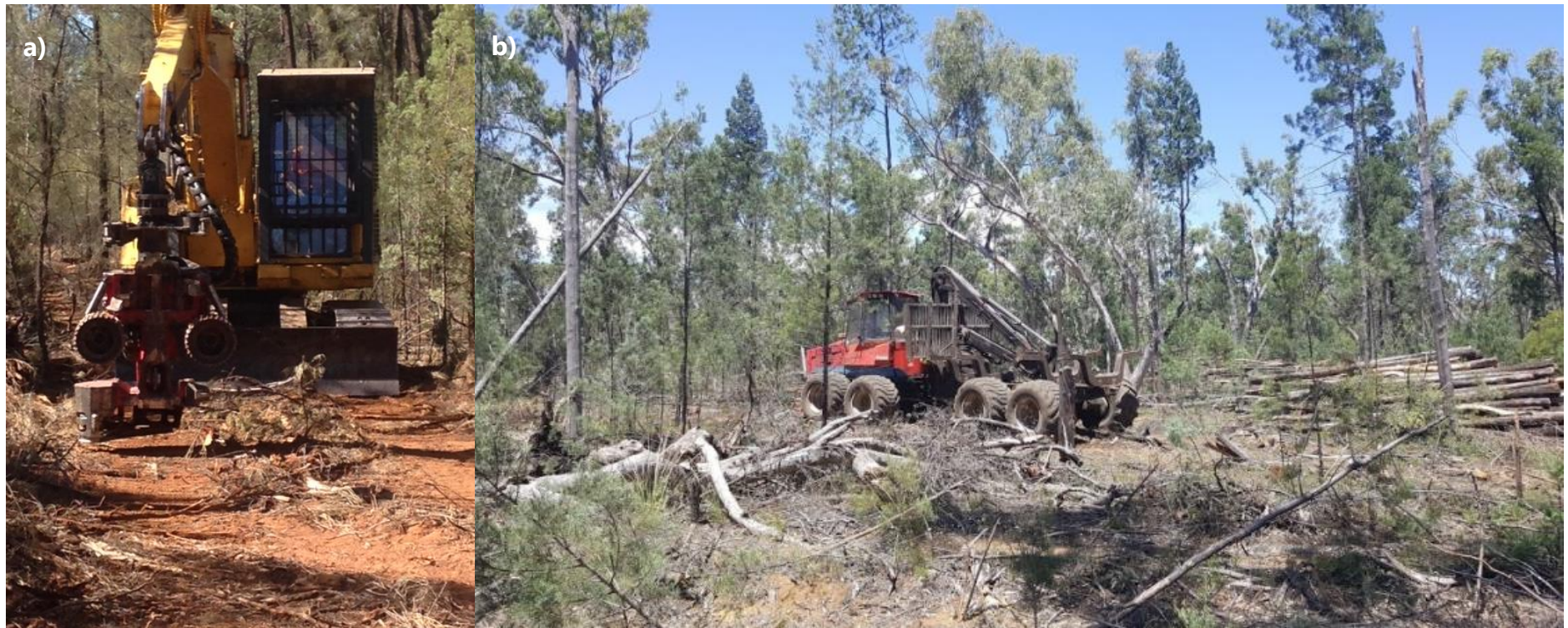
Fig. 3.2.2. A small mechanized harvester used in an early thin site (a) and a forwarder used in a second thin site to remove the stock pile of stems (in background) from the forest (b).
