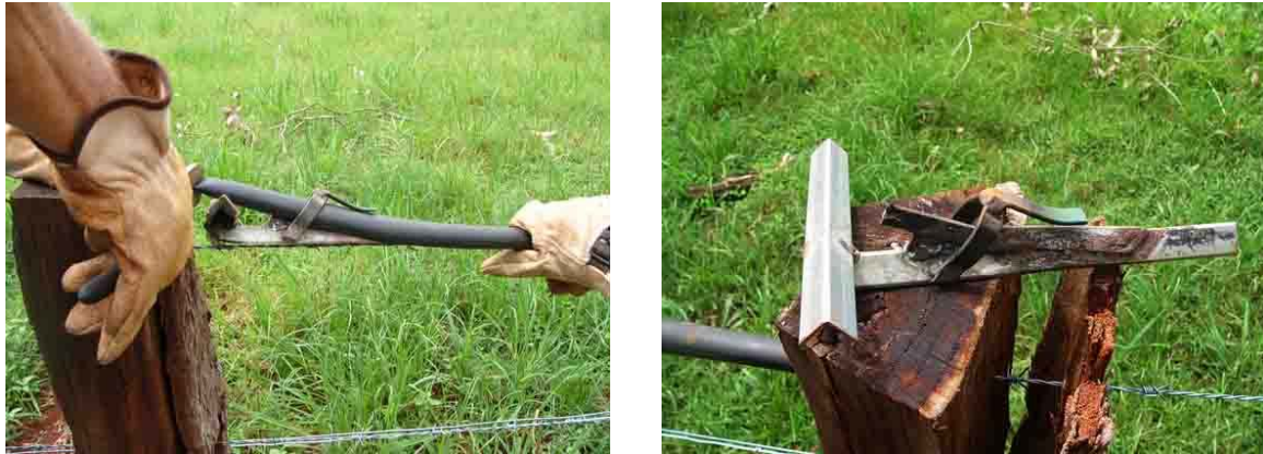
Fig. 1 The polypipe splitter device that simultaneously splits and installs the pipe over barbs.
