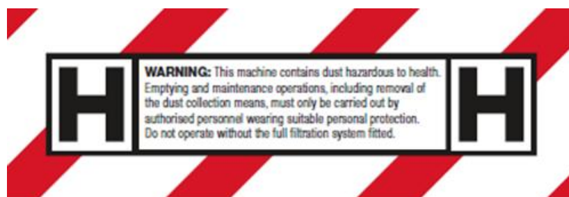
Figure 11: Hepa filter warning label
