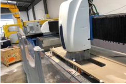
Figure 4: CNC Router with plastic shrouding. Source – WHSQ Inspectorate
