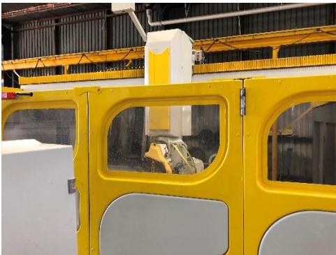
Figure 5: An example of isolation, with workers outside of the barrier. Source – WHSQ Inspectorate
