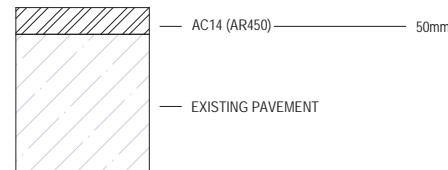
PAVEMENT TYPE 6 MILL AND RE-SHEET - LOCAL ROADS SCALE 1:10
