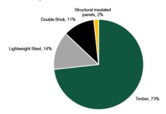
Figure 6 Load Bearing Elements in New Detached Houses
