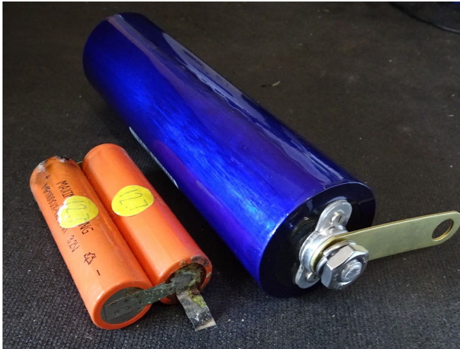
Small format welded throw away cells (left) vs. large format threaded terminal replaceable cell as used in government batteries.
