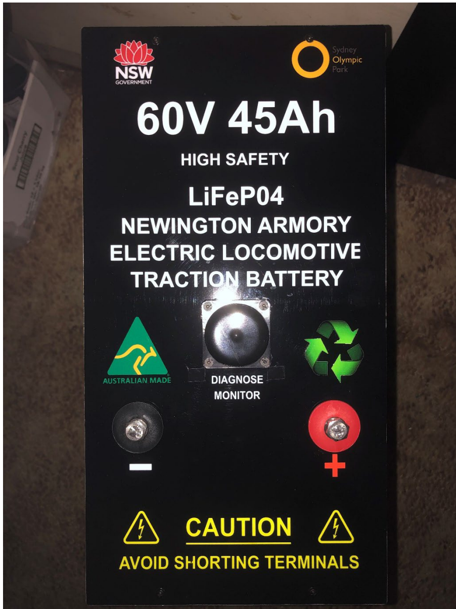
Transport for NSW- Sydney Olympic Park locomotive battery
