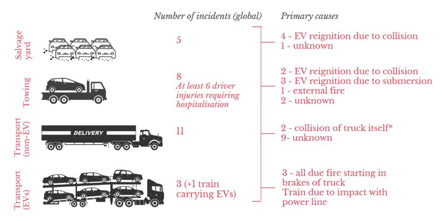
\*In transport of non-EV LiBs trucks were carrying; 1 x e-motorbikes, 2 x Tesla battery packs, 2 x emopeds/scooters & 5 x assorted smaller LiBs (phone, laptop, vapes etc)
