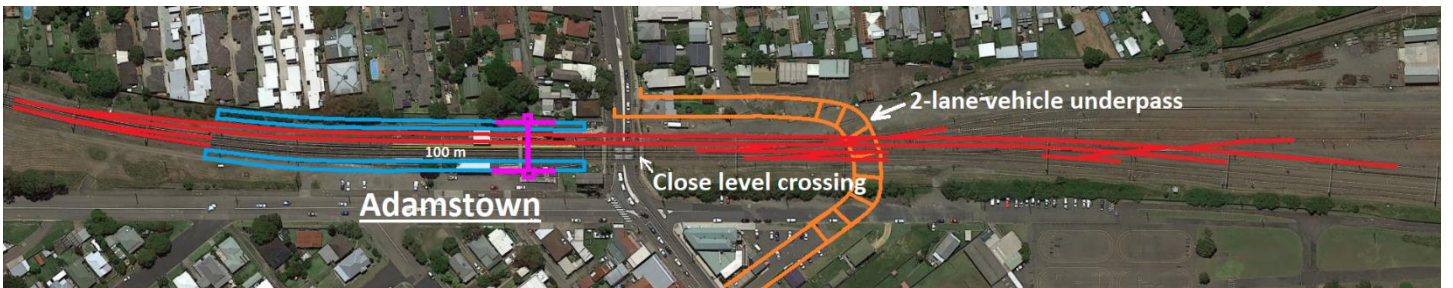
Adamstown level crossing closure post construction of a road underpass with pedestrian crossing via station access
