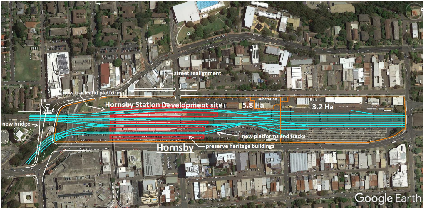
Hornsby Station – extra platforms and site development with heritage building preservation
