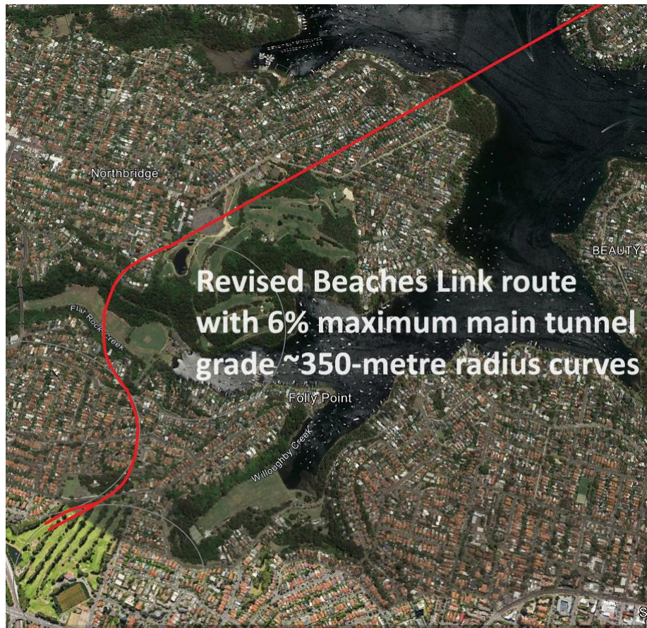
Figure 4: Beaches Link revised route with ~6% main tunnel grade and ~350-metre radius curves under cammeray and Tunks Park
