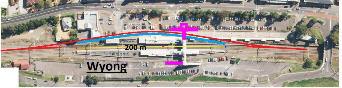
Wyong – new platform to create double-island platforms
