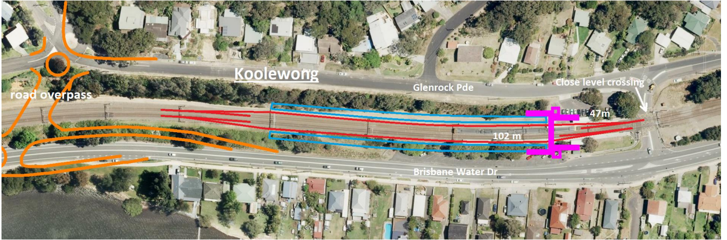
Koolewong road over pass and level crossing closure
