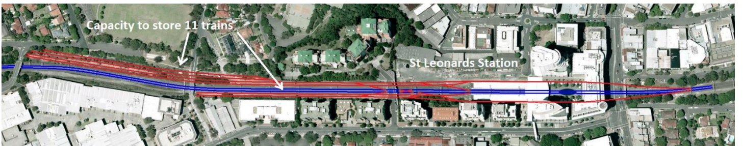
Figure 6.2 - St Leonards Station turnback to replace Lavender Bay train store (stabling yard)
