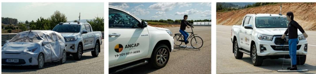
Figure 9 - AEB Scenarios: Car-to-Car rear, Car-to-Cyclist and Car-to-Pedestrian
