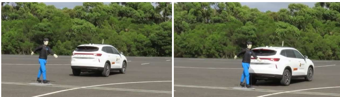
Figure 13 – Reversing (back over) Testing
