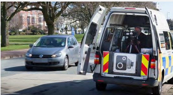
Figure A.7: Ireland: Highly overt MSC vehicle with no signs (but with warning decals)
