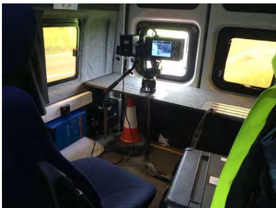
Figure A.21 UK: View of the Camera operator position from within a new 'Long Ranger' MSC van.
