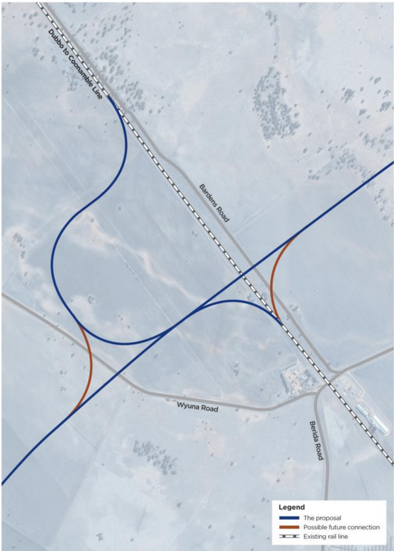
Figure 9 - Intersection between the Inland Rail Study Area and existing line near Curban (suggested connection shown in red)
