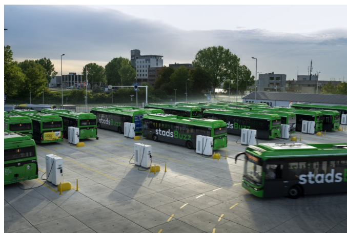
Figure 6 – Electric bus charging at a depot in Dordrecht, Netherlands – the second city in the country to convert to 100% electric. Source: https://www.ebusco.com/charging/
