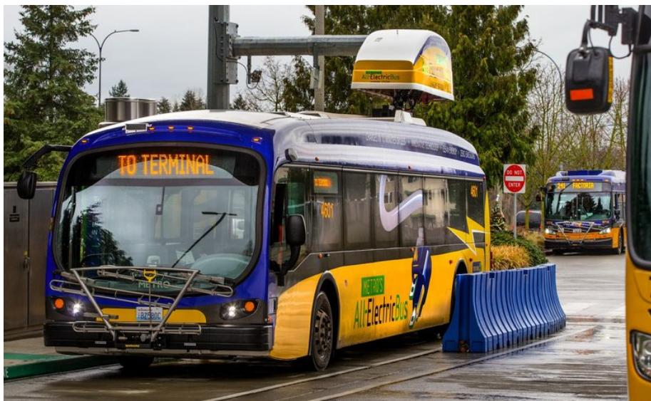
Figure 22 - One of KCM's electric buses using an overhead, fast-charger during a layover.
