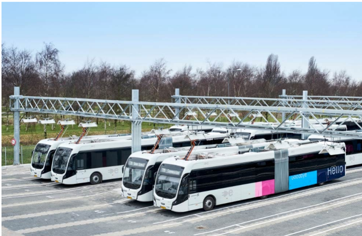
Figure 28 - Electric buses at Schiphol charging using overhead pantograph chargers. Source: https://www.schiphol.nl/en/schiphol-group/page/europes-largest-fleet-of-fully-electric-buses/
