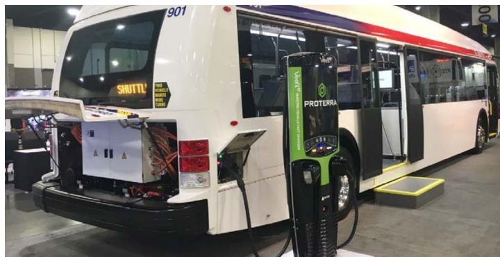
Figure 5 – Australian-built Tritium DC fast-charger being used to charge an electric bus in the US. Source: https://www.electrive.com/2019/03/12/india-tritium-signs-deal-with-tata-to-supply-dc-chargers/
