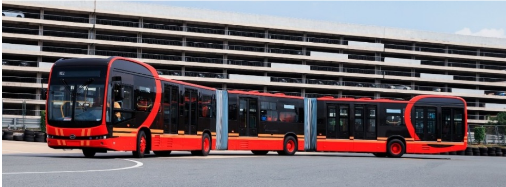
Figure 1 - The BYD K12A is an electric bus capable of carrying up to 250 passengers, with a driving range of 300 kilometres. Source: https://newatlas.com/byd-world-longest-electric-bus-k12a/59179/
