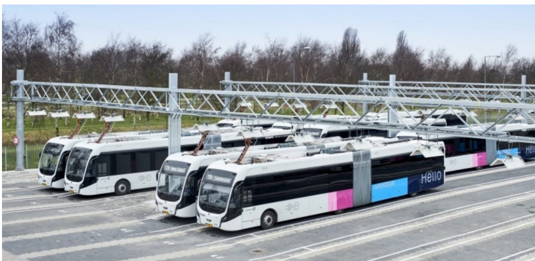
Figure 7 – Electric buses charging using overhead pantograph chargers at a bus depot in Schiphol in The Netherlands.
