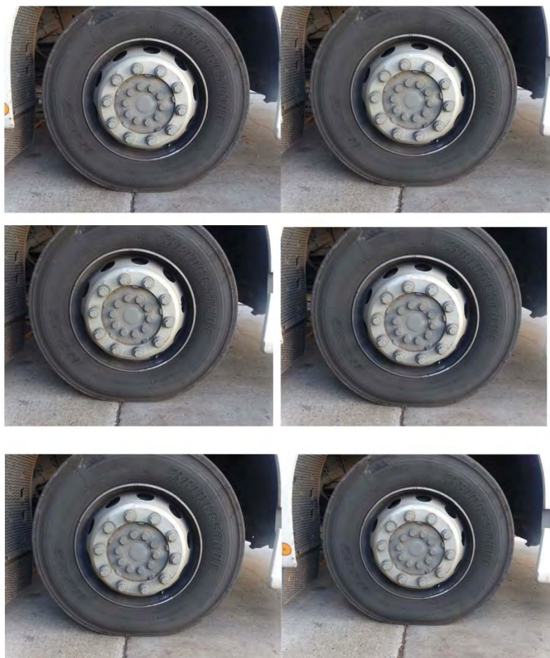
Figure 1; 295/80R22.5 steer tyre, reduced by 10 psi from 120psi to 60psi. When is it flat?
