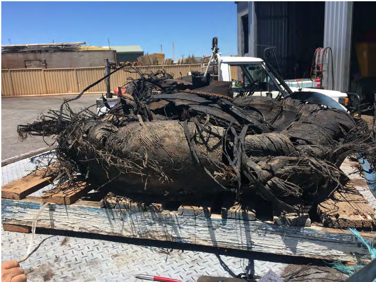
Figure 3; catastrophic steer tyre failure, how do you evidence the pressures were appropriate?
